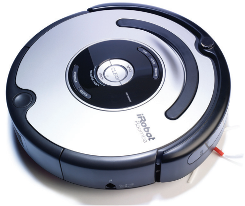
FIGURE AP1.6 A robotic vacuum cleaner communicates with the base station as it maneuvers around the room. (Photo courtesy of Hugh Threlfall/Alamy.)
