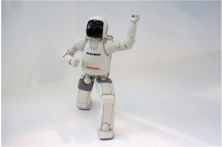
FIGURE 1.12 The Honda ASIMO humanoid robot. ASIMO walks, climbs stairs, and turns corners. (David Coll Blanco/Alamy Stock Photo)
