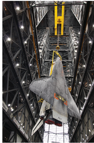
FIGURE AP2.6 (a) Hanging crane supporting the Space Shuttle Atlantis (photo courtesy of: NASA/ Jack Pfaller) and (b) schematic representation of the hanging crane structure.
